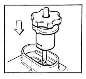
6. Place the collet assembly over drill and locate the flat faces on the collet holder with the flat faces on the sharpener body by turning the holder CLOCKWISE only, and NOT twisting. Then push firmly down.
