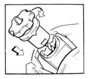
8. Insert the collet/drill assembly into swivel guide and switch on power. Place fingers over locknut and grip collet holder – do not turn assembly using locknut. Using slight downward pressure and following the cam action. Rotate the assemt through a complete circle of 360° several times. Your MARTEK sharpener will remove approx. 0.015° from the drill – more than sufficient to sharpen most bits.
