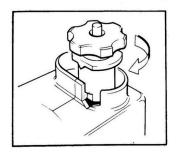
7. Tighten the collet locknut until the drill is held firmly but do not over tighten. You can now release the drill clamp and remove the assembly complete with drill ready for sharpening. Whilst tightening the locknut keep downward pressure on top of the drill bit, as a loose locknut can let the drill move about. This will ensure that the drill bit is maintained at the correct depth setting.
