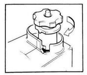
7. Tighten the collet locknut until the drill is held firmly but do not over tighten. You can now release the drill clamp and remove the assembly complete with drill ready for sharpening. Whilst tightening the locknut keep downward pressure on top of the drill bit, as a loose locknut can let the drill move about. This will ensure that the drill bit is maintained at the correct depth setting.
